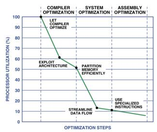
Figure 4. Steps in optimizing Vorbis source code on Blackfin, leading to significantly reduced processor utilization.
