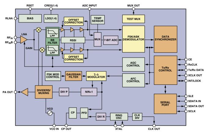
Figure 2. Functional block diagram of the ADF7020.
