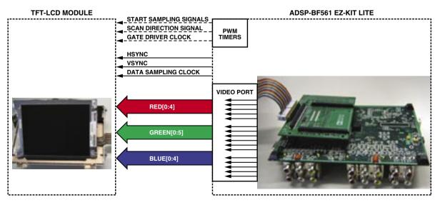
Figure 1. 5-6-5 LCD connection: The ADSP-BF561 eliminates the need for a timing ASIC by supplying the dotted-line connections.
