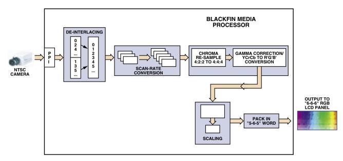
Figure 2. Example of system flow: converting a signal from a camera source to an LCD display output.
