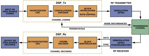
Figure 3. Signal-processing functions.
