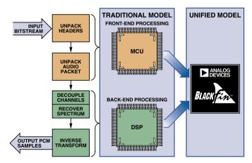
Figure 2. Generalized processor flow for the Vorbis decode process.
