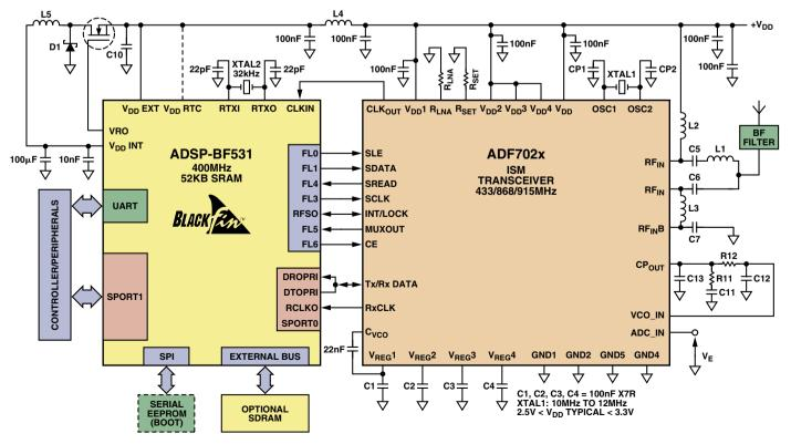
Figure 1. Circuit diagram of the modem.
